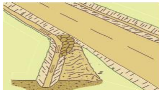
Figure 3-2 Mitre-drain diverting water from main road side drain, to a stable area, and into storage or recharge structures
