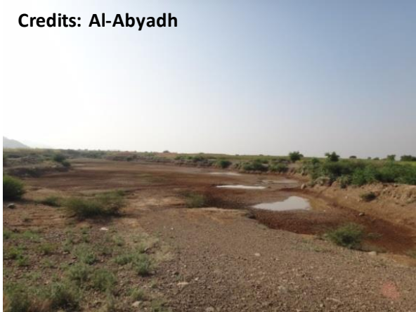
Photo 3.16 Using a borrow pit in Wadi Tabab near the road as retention and recharge pond (left)
